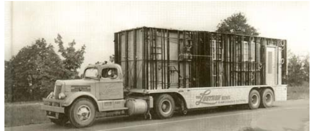
Figure #6 - Lustron flatbed trailer for transporting house to site.
